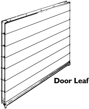
Wind load is transferred to the vertical guide rails by the horizontal aluminum beams of the door leaf. These beams hang between two continuous sheets of vinyl-coated polyester fabric, thus pulling the fabric tight and stabilizing the beams. Self-lubricated guide blocks travel in the guide rails at each end of the door leaf beams.
